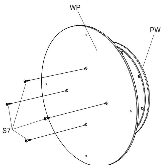
**1. Mount the wheel and wall plate to wall**
